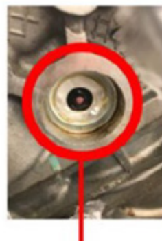
Overheated Red Sensor +255°F Coolant Temp
