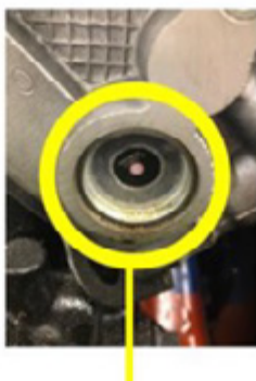
Overheated Pink Sensor 255°F Coolant Temp
